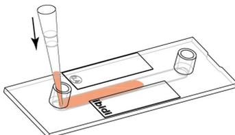
In special cases, e.g. when the channel surface is hydrophobic or when filling small channels, it might be necessary to fill the channel with a syringe. Use a low volume syringe with 1 or 2.5 ml!
